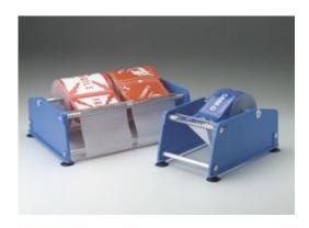
Label caddies look and work much like a tape dispensers. A roll of labels is inserted into the unit and threaded through a set of rollers. When the label is pulled, the label is stripped from the liner for easy grab and stick application.
